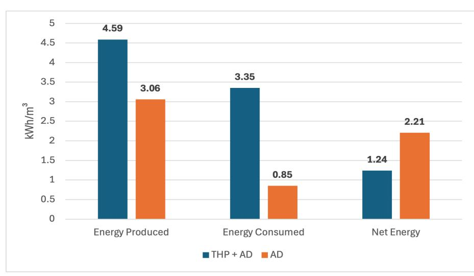
THP + AD required more input energy than AD alone due to the additional pretreatment stage. Despite this, THP significantly boosted biogas production, improving the overall energy recovery potential of the system. This trade-off demonstrates how higher upfront energy use can still lead to greater long-term energy efficiency.
