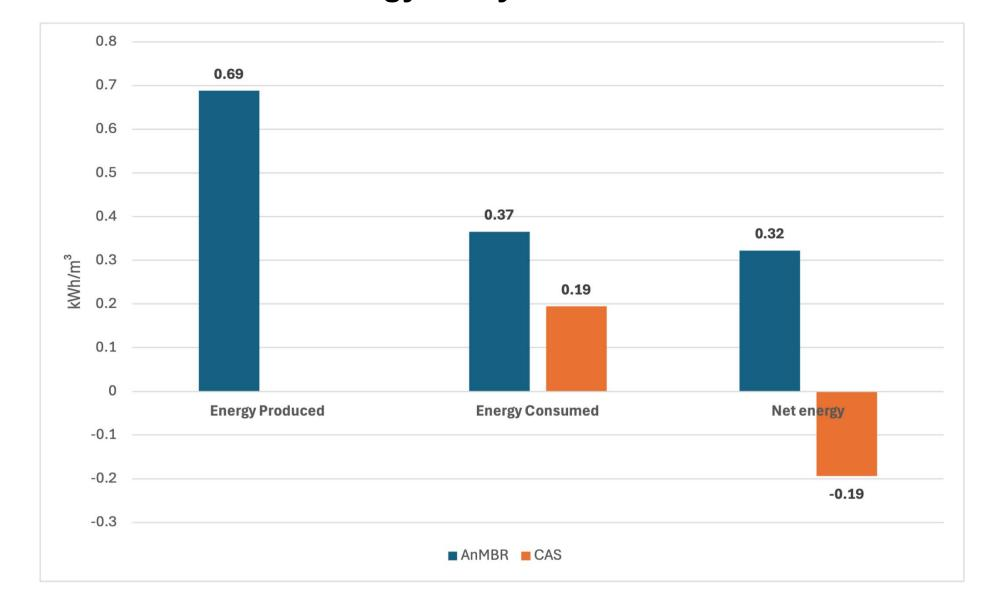
AnMBR consumed more electricity per m³ of wastewater (0.37 kWh/m³) compared to the Conventional Activated Sludge (CAS) process (0.19 kWh/m³). However, AnMBR generated energy-rich biogas, resulting in a positive net energy balance, while CAS remained entirely energy-negative. This highlights AnMBR's advantage as a more sustainable option when resource recovery systems are optimized.
