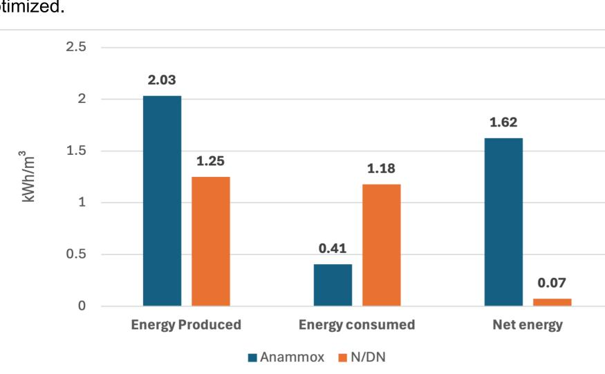
Anammox reduced energy use by approximately 65% compared to the traditional nitrification/denitrification (N/DN) process. This reduction comes mainly from eliminating the aeration step, which is highly energy-intensive in N/DN. The result makes Anammox the most energy-efficient option among the technologies studied.
