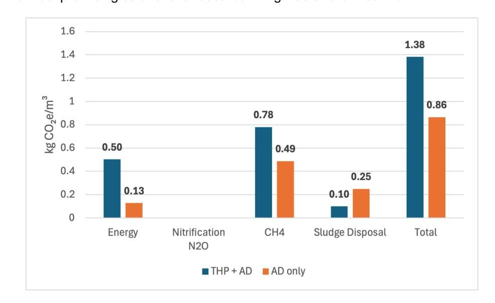
THP + AD lowered sludge-related emissions compared to AD alone, as the process reduced biosolids volumes and improved digestion efficiency. It also helped limit methane slip by improving gas recovery. If paired with renewable energy for its heat and electricity needs, THP + AD could achieve even greater reductions in overall carbon footprint.
