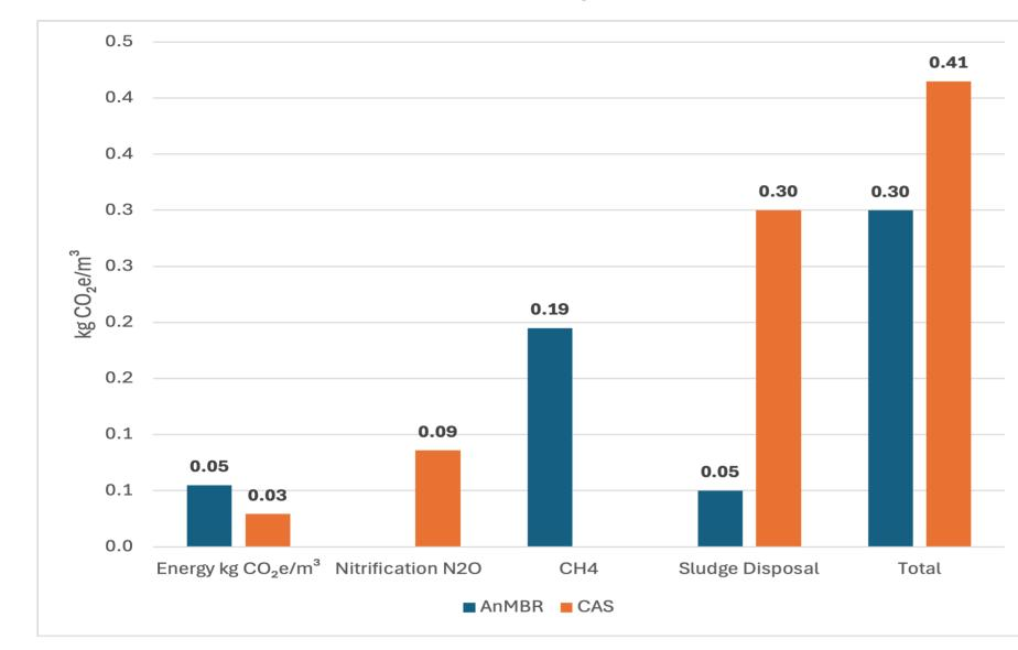
AnMBR produced fewer overall emissions than CAS because it required less aeration and reduced sludge volumes. While CAS emissions were dominated by sludge disposal, AnMBR's main risk was methane leakage during operation. Proper methane capture technologies are therefore critical to maximize AnMBR's climate
