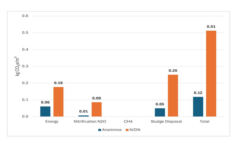
Anammox achieved the lowest GHG emissions profile of all technologies evaluated. This was due to the elimination of nitrous oxide emissions typically associated with nitrification and denitrification, combined with reduced electricity demand. Its dual advantage of energy savings and lower emissions makes it one of the most promising solutions for decarbonizing wastewater treatment.
