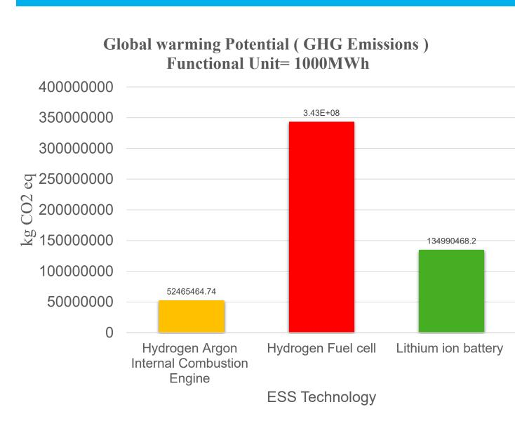
HAICE shows the lowest manufacturing emissions and avoids NOx pollutants from hydrogen combustion, while fuel cells and lithium-ion batteries have higher GWP due to material intensity, especially platinum-group metals and battery metals. Operational emissions are negligible except in hydrogen-based systems, where GWP depends on hydrogen production methods and system efficiency.
