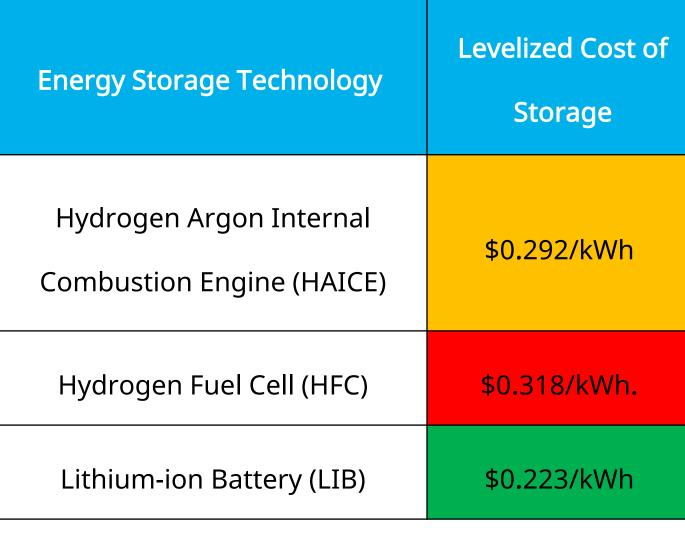
Lithium-ion batteries (LIB) have the lowest levelized cost of storage (LCoS), with balanced contributions from capital and electricity charging costs.
