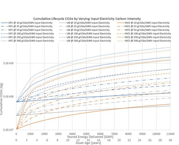
Life cycle CO2 emissions show HFC systems have the highest emissions due to construction intensity and low RTE, while HICE starts lowest but surpasses LIB emissions after ~20 years; improving HICE efficiency can maintain lower emissions long-term. Emissions for all technologies rise with input electricity carbon intensity, but LIB's higher RTE results in slower cumulative emissions growth compared to hydrogen systems reliant on electrolysis.
